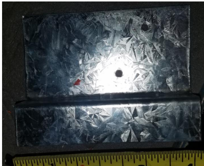
Short Z-track, secured to horizontal tracks, to secure each panel
